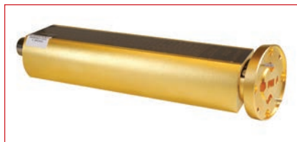
▲ Fig. 2 Noise source STZ-05267313-VM-02 operates from 40 to 60 GHz and has a UG-383/U-M anti-cocking flange.
