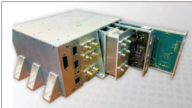
▲ Fig. 2 LISA charge management device prototype. Source: University of Florida.
